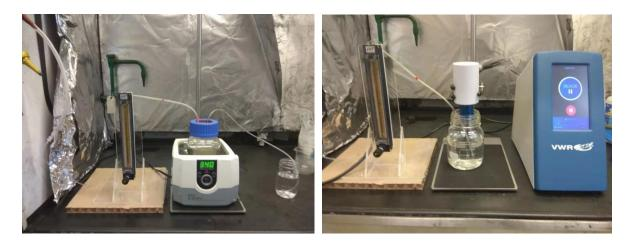
Figure 4. PFAS Sonochemical Degradation Experimental Setup
