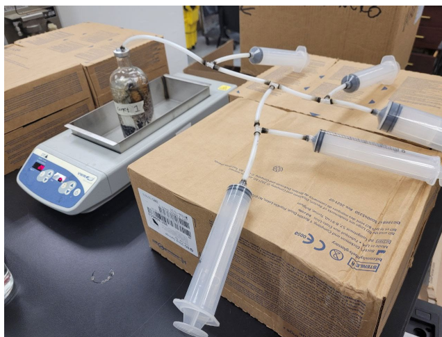
Figure 5. Set-up of a bottle for evaluating the fate of PFAS in solid waste
