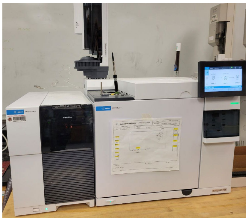
Figure 2. Equipment (i.e., gas chromatography - mass spectrometry) for measurement of FTOHs
