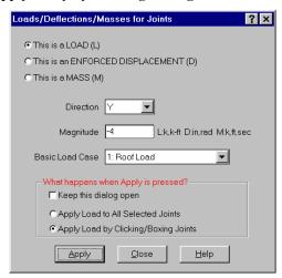
We will use this to apply loads to the interior joints on the top of the trusses and apply loads of different magnitudes to the outer joints.
