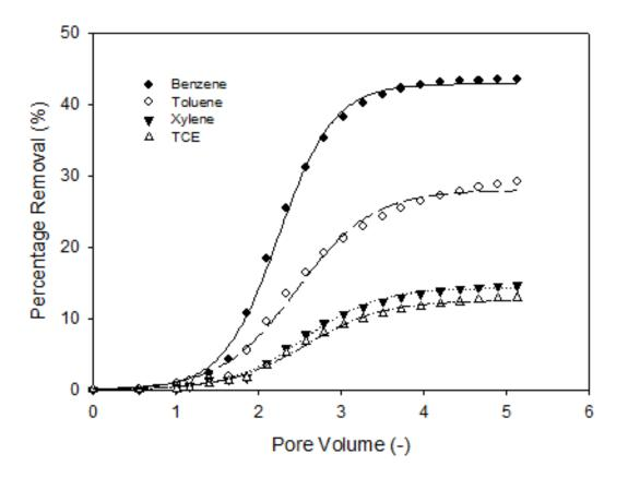
Figure 13. BTEX and TCE Removal by Adsorption
