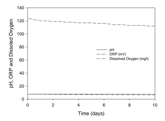
Figure 11. pH, ORP and Dissolved Oxygen during Benzene Degradation
