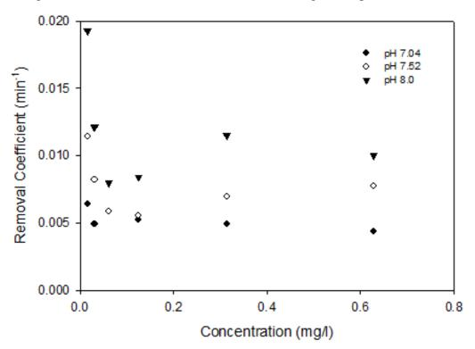
Figure 18. Iron Removal Coefficient against pH and Input Concentration
