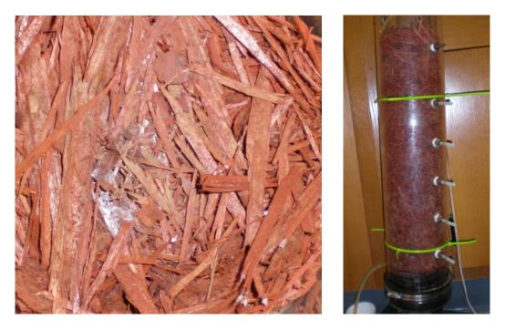
Figure 4. Mulch (Left Image) and Biofilter with Mulch as the Filter Media (Right Image)
