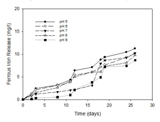
Figure 26. Ferrous Iron Release for Franklin County
