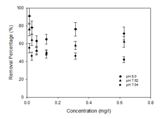
Figure 16. Iron Percentage Removal against pH and Input Concentration
