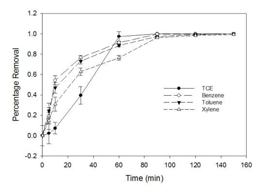
Figure 9. BTEX and TEC Percentage Removal by Evaporation
