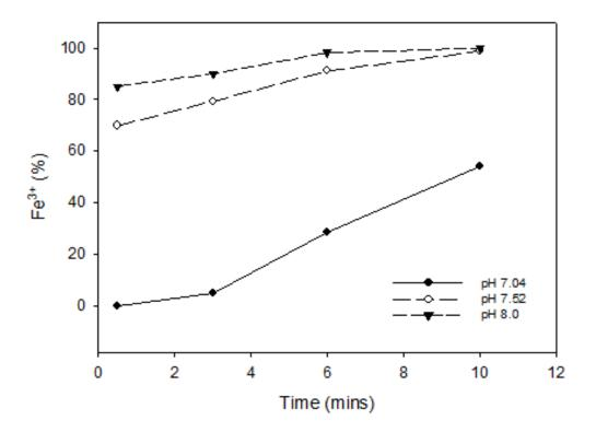
Figure 14. Ferrous Iron Oxidation as a Function of pH and Reaction Time
