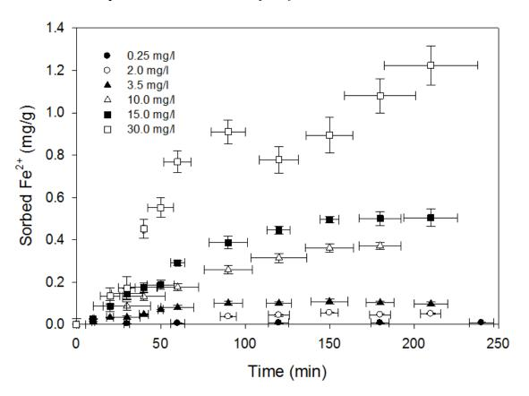
Figure 21. Ferrous Iron Kinetic Adsorption on S. putrefaciens
