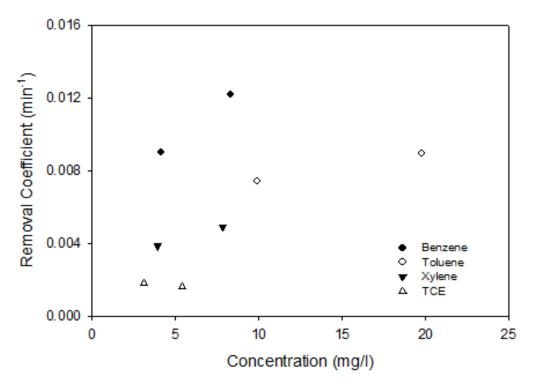
Figure 17. BTEX and TCE Removal Coefficient against Input Concentration
