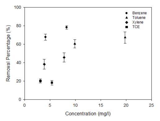
Figure 12. BTEX and TCE Percentage Removal during Water-Filled Trench with Biofilter
