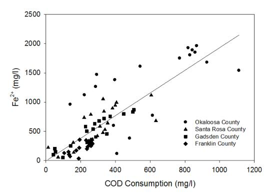
Figure 20. Ferrous Irion Release with Landfill Leachate Decomposition
