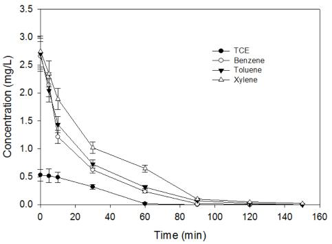
Figure 8. BTEX and TEC Removal by Evaporation
