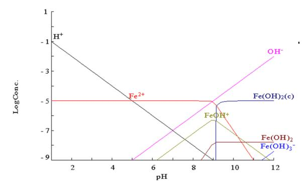
Figure 22. Ferrous Iron Speciation as a Function of pH
