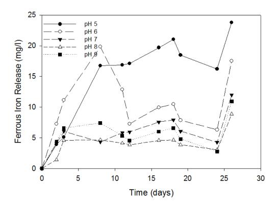
Figure 23. Ferrous Iron Release for Okaloosa County
