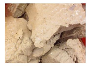
Figure 1. Alum Sludge Collected from Atlanta-Fulton Water Treatment Plant
