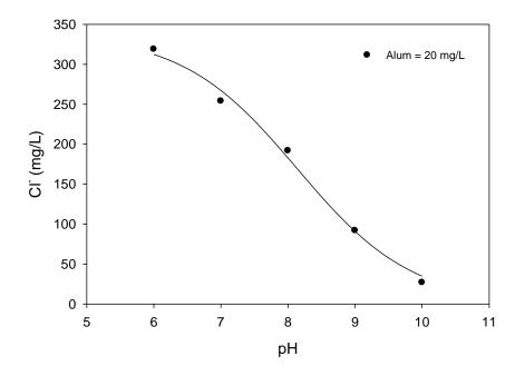
Figure 3. Residual Chloride Concentration as a Function of pH
