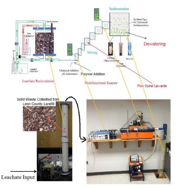
**Figure 1. Experimental Setup of This Research**
