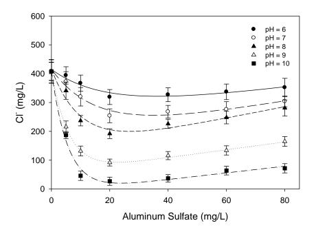
Figure 2. Chloride Removal as a Function of Alum Concentration
