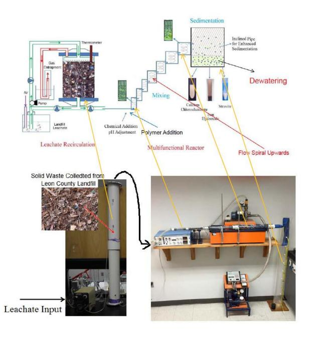
Figure 1. Experimental Setup of This Research
