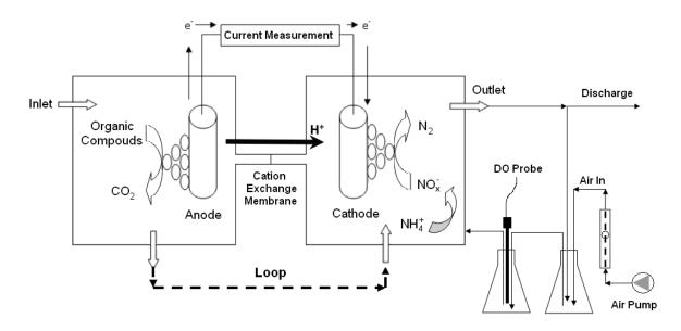
Figure 1. MFC/Anammox Reactor Setup
