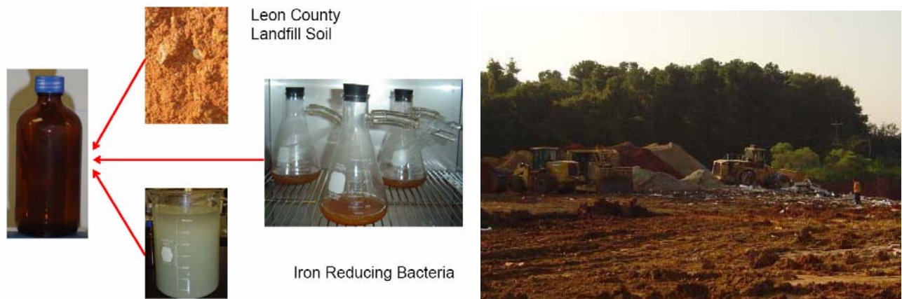
Figure 3. Laboratory Iron Reduction Experiments Using Soil Collected from Leon County Landfill (Left) and Site Picture of Leon County Landfill (Right)
