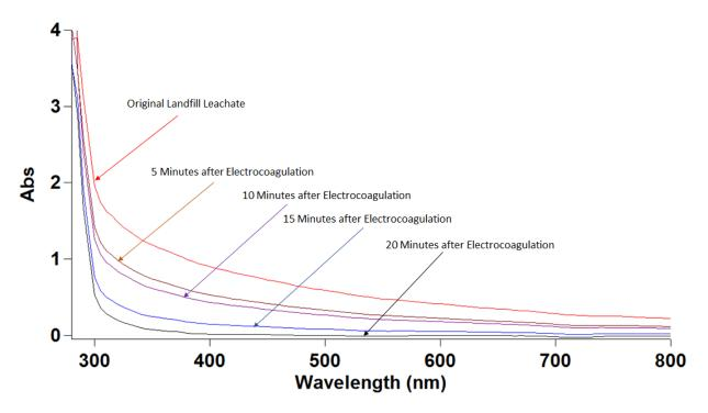
Figure 2. Leachate UV-Vis Spectrum after Electrocoagulation
