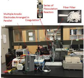
Figure 1. Experimental Setup of This Research
