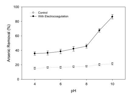
Figure 3. Arsenic Removal by Electrocoagulation as a Function of pH
