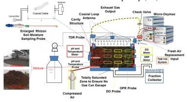
Figure 1. Experimental Setup
