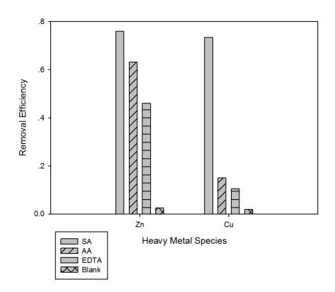
Figure 1. Cu and Zn Extraction from Granular Sludge Pellet SA: Sulfuric Acid, AA: Acetic Acid
