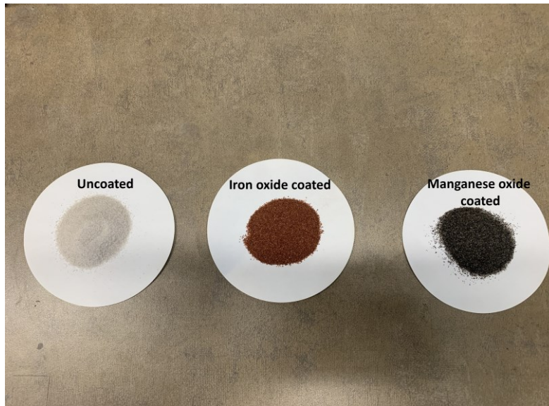
Figure 9. Uncoated Sand, Iron Oxide-Coated Sand and Manganese Oxide-Coated Sand
