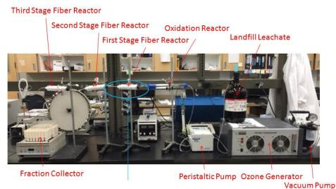
Figure 1. Experimental Setup
