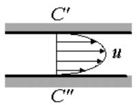
At and beyond station C the flow is called developed. We will assume that the flow is nonturbulent and that the streamlines have become parallel. These assumptions allow us to solve the incompressible Navier-Stokes equations exactly!
