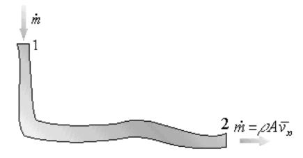
Note that according to continuity,  $\dot{m}$  is constant, so that the average velocity v increases when S becomes smaller.
