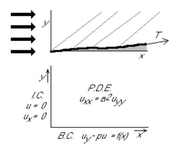
Figure 2: Supersonic flow over a membrane.
