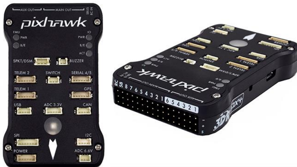
Figure 6 - Flight control hardware - Pixhawk [6]
