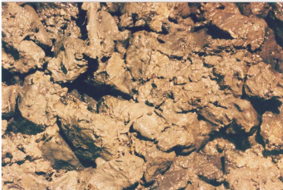
Fig. 17. Drainage stone in mesocosm after 20 months exposure to leachate.
