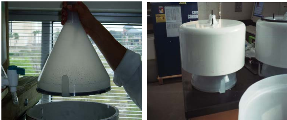
Figure 3. Leachate Application System Consisting of Inverted Funnel and Perforated Plate.
