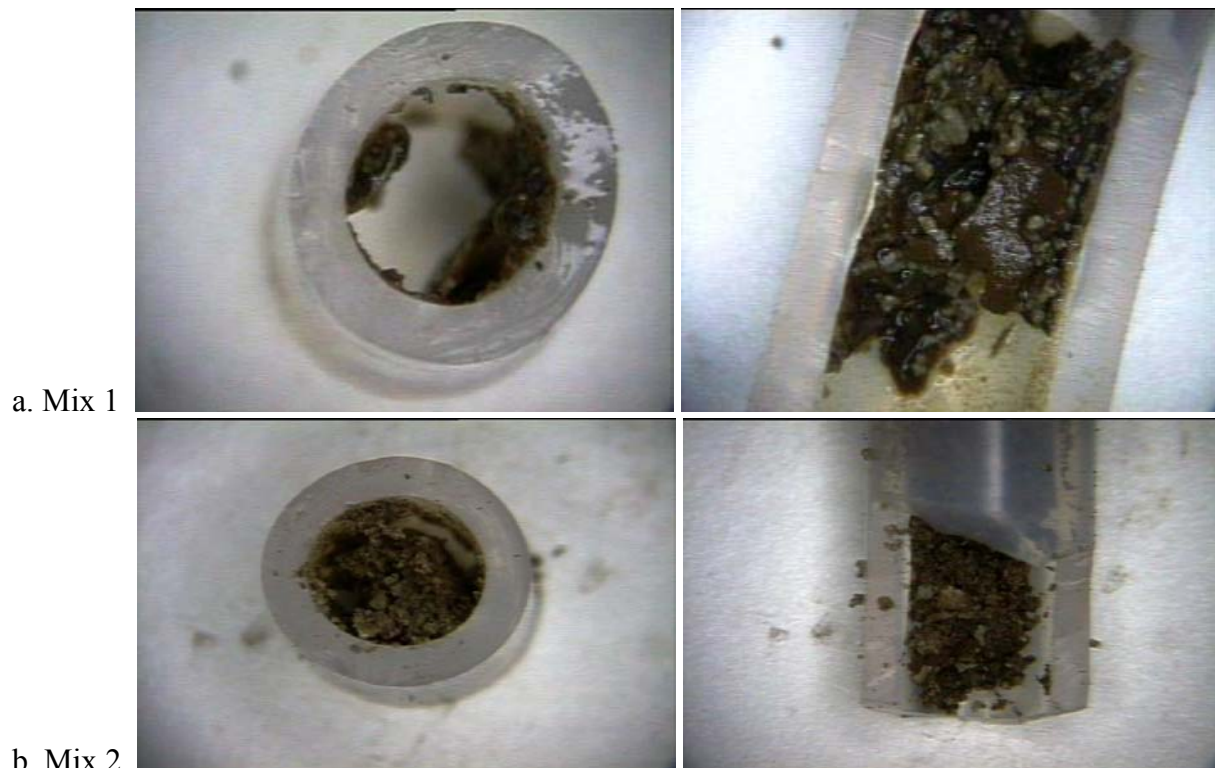
Figure 28. Photograph of deposits in leachate collection tubing from a.) Mix 1 and b.) Mix 2. The tubing has an ID of 8 mm and OD of 10 mm.
