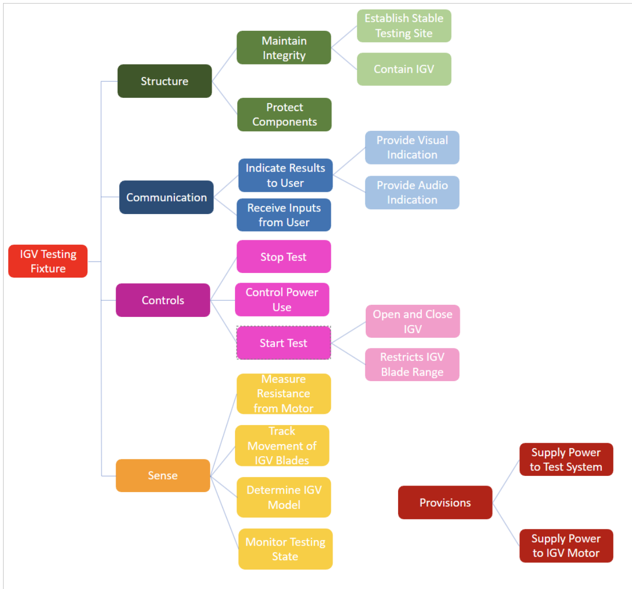
Figure 2 Functional hierarchy denoting the flow of the functions.
