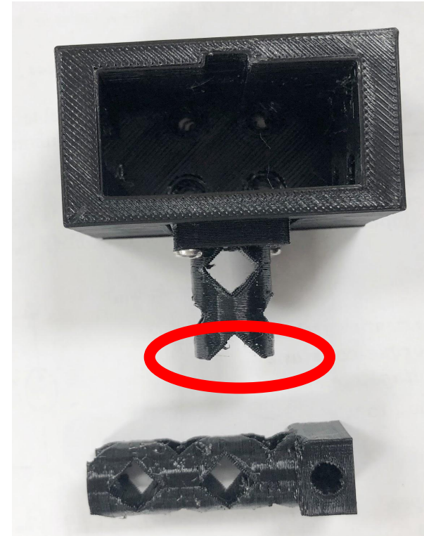
Figure 2. Second broken linkage attached to motor mount.
