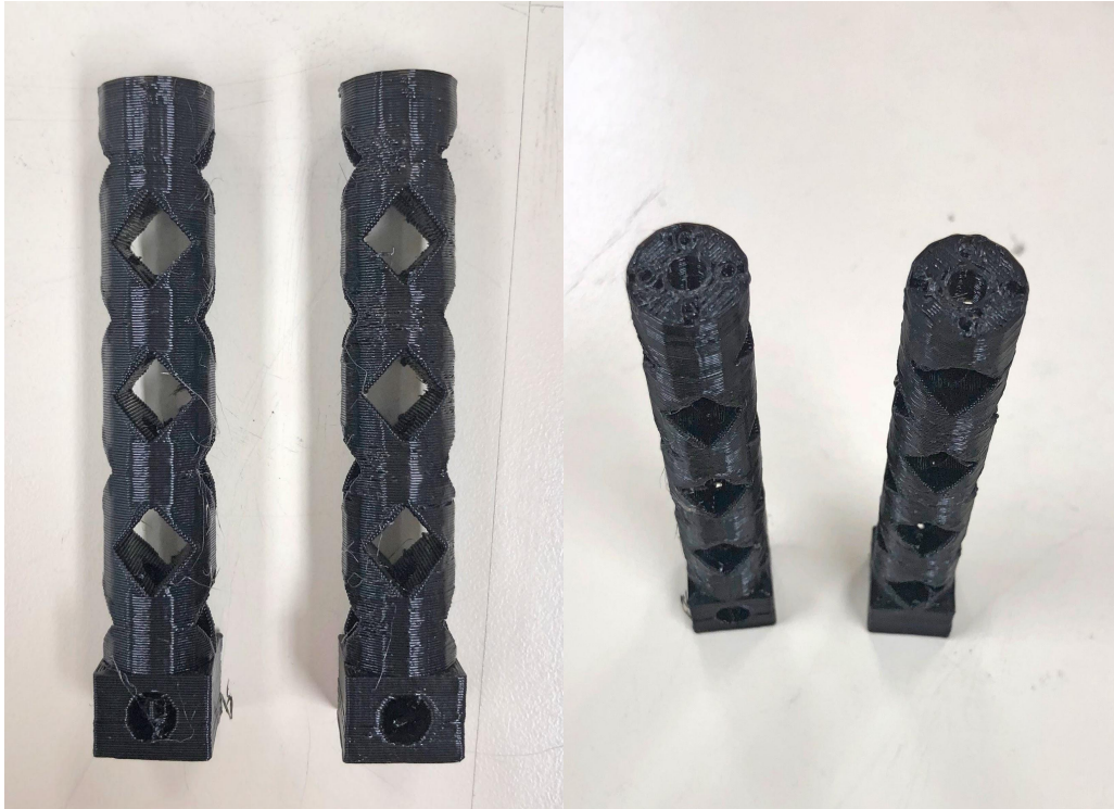
Figure 1. 3D printed linkages.
