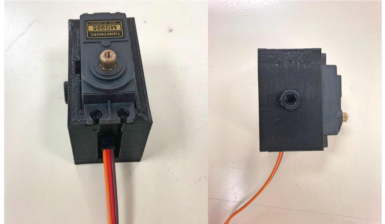
Figure 2. Servo motor in motor in 3D printed motor mount.
