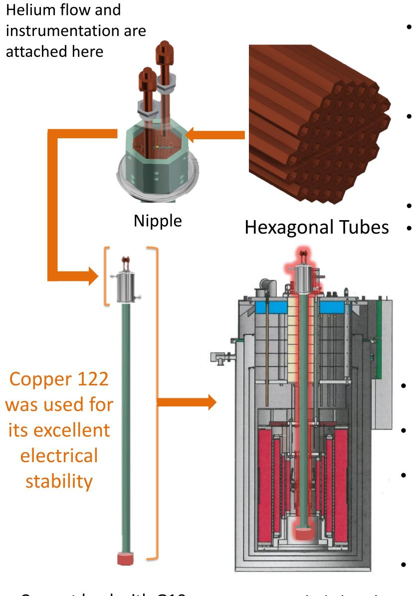
Current lead with G10 Insulation (green) and test coil (red)
