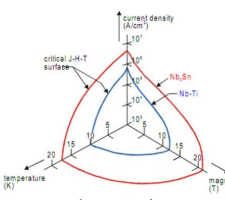
Superconductivity means zero electrical resistance in a material and depends on a current density(J), temperature(T) and
