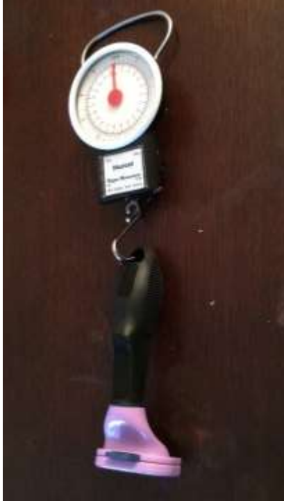
Figure 8: Required Manual Brushing Force Test
