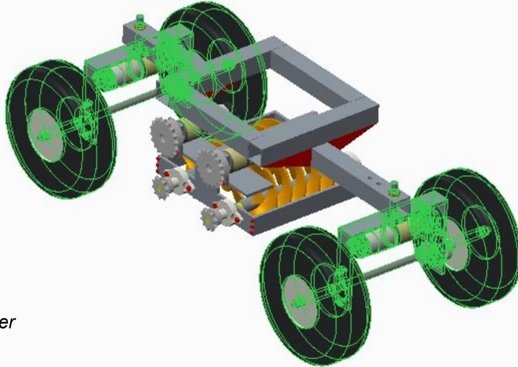
**Figure 7:** *Robo-Weeder with Highlighted Drive Mechanism.*
