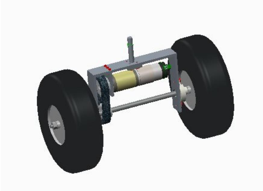
*Figure 8: Robo-Weeder Drive Mechanism.*
