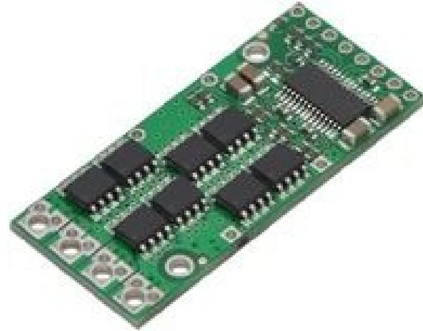
*Figure 11: Motor Driver for use on the Robo-Weeder.*
