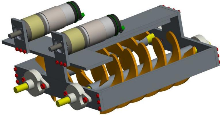
*Figure 10: Fully Assembled Shearing Mechanism.*
