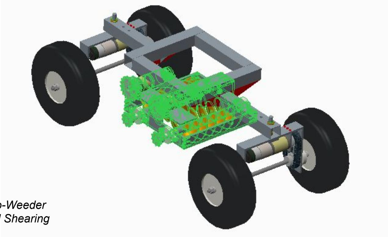
**Figure 3:** *Robo-Weeder with Highlighted Shearing Mechanism.*
