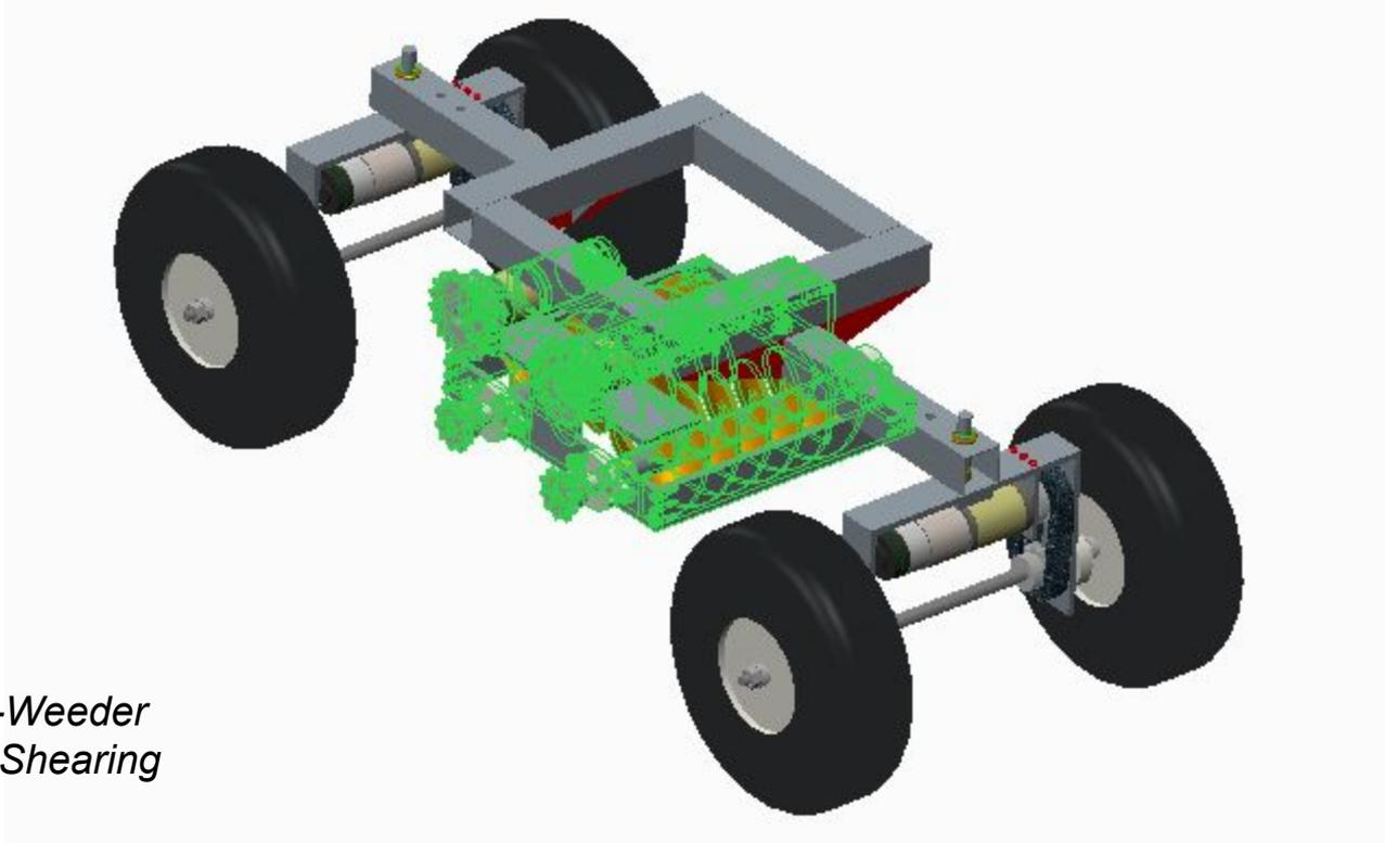
**Figure 9:** *Robo-Weeder with Highlighted Shearing Mechanism.*
