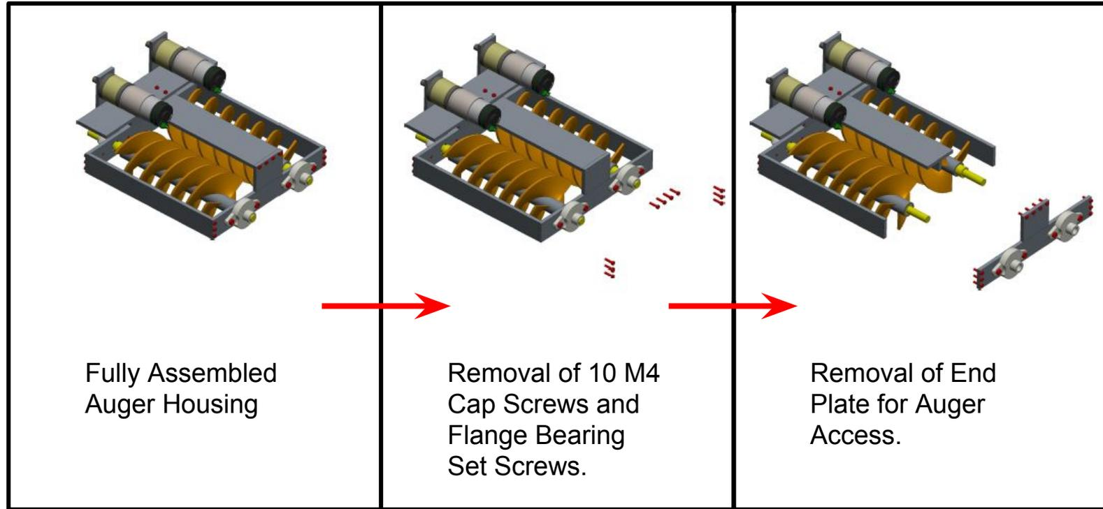
*Figure 6: Illustration showing the removal of the Auger Assembly.*
