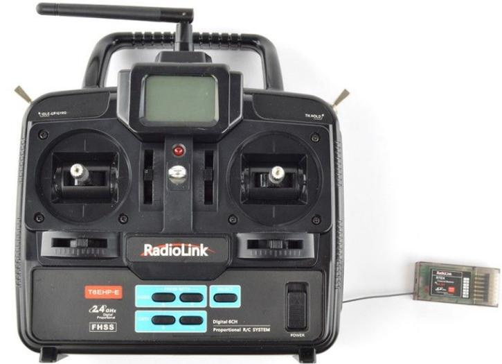
**Figure 9:** Robo-Weeder Transmitter and Receiver.
