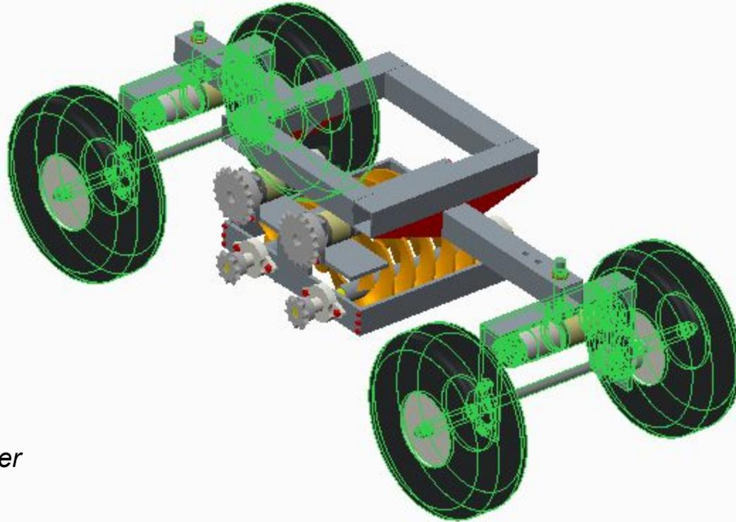
**Figure 7:** Robo-Weeder with Highlighted Drive Mechanism.
