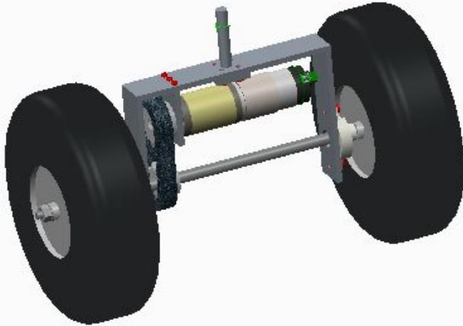
*Figure 8: Robo-Weeder Drive Mechanism.*
