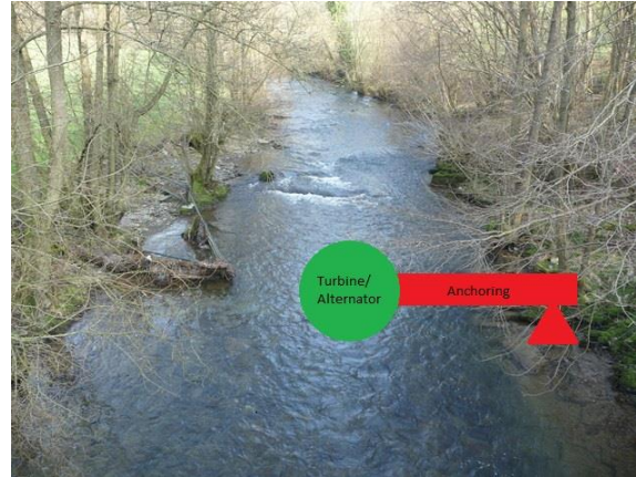
Figure 14 - Cantilever style anchoring system
