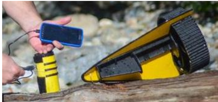
Figure 2 - StreamBee, powers small electronic devices with a USB port
