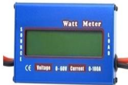
Figure 14 - LCD Digital 60V/100A Watt Meter
