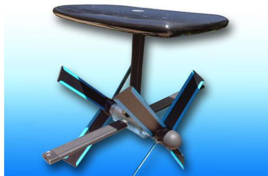
Figure 2 - Back Pack Power Plant: 3 feet in length and weighs 30lbs
