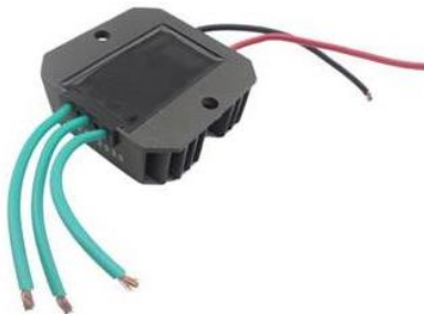
Figure 13 - 12 Volt 25 Amp Charge Controller
