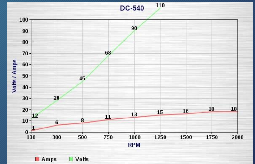
Figure 24 - Production Based on RPM (Based on OC and SC)
