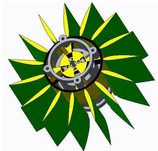
Figure 6: Current airfoil-blade fan design
