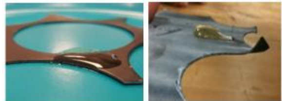
Figure 19. Rubber coated metal gaskets before and after application of oleophobic solution.
