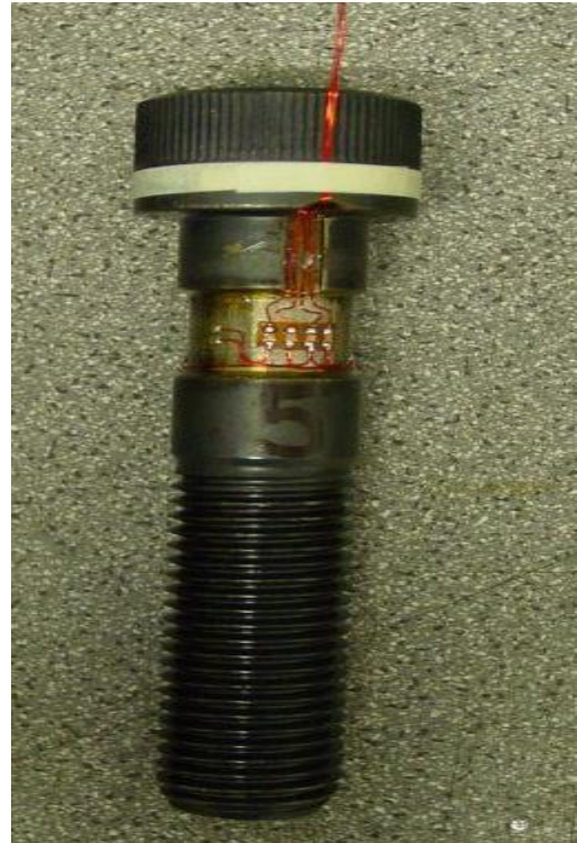
Figure 13. Modified bolt with strain gauge.
