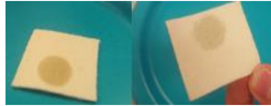
Figure 20. High density felt after oil has been poured onto it.
