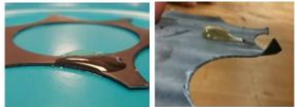
Figure 27. Rubber coated metal gaskets before and after application of oleophobic solution.
