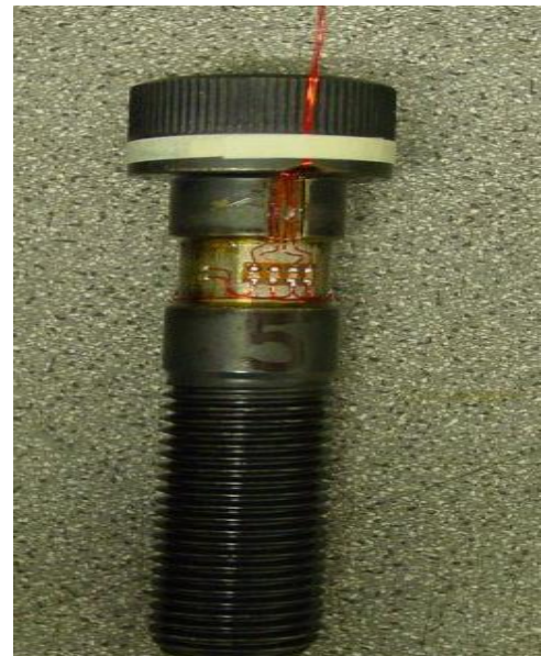
Figure 14. Modified bolt with strain gauge.
