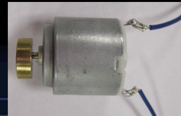
Image 17 : DC vibration motor of 7,100 rpm.
