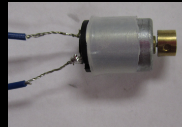
Image 16 : DC vibration motor of 4,500 rpm.
