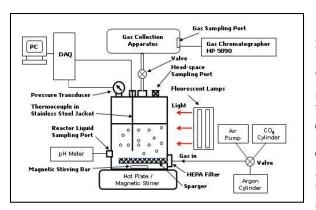
Figure 2: Schematic of a Photobioreactor.
