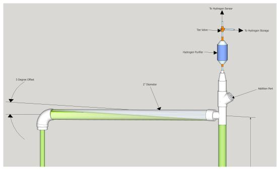
Fig 3A: Top half of photobioreactor.
