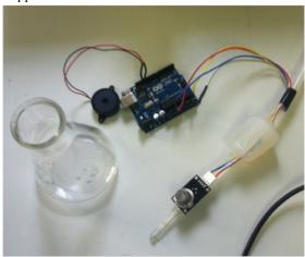
Fig 5: Prototype of H2 sensor system.
