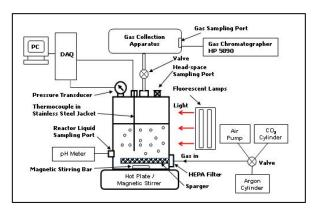
Fig 2: Schematic of a Photobioreactor.
