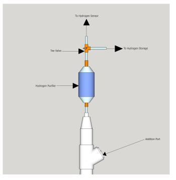
Fig 2A: Components and connection of degasing column.
