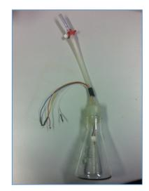
Fig 6: Airtight beaker with sensor.
