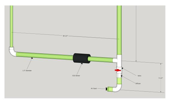
Fig 4A: Top half of photobioreactor.
