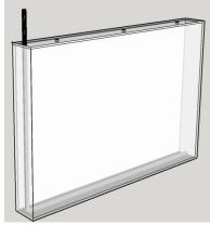
Figure 5: Flat Plate Bioreactor
