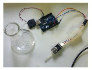
Figure A: Prototype of H2 sensor system.
