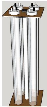
Airlift and flat plate bioreactors are advantageous systems because they use compressed air to mix as well as control the temperature of the system. This results in a more efficient NER.
