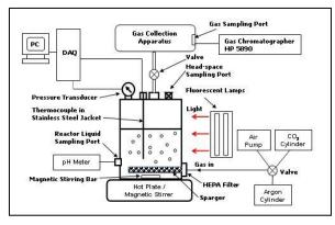
In order to produce  $H_2$  from algae, the algae must be cultivated in a controlled manner. There are two ways to cultivate algae: open ponds and photobioreactors. Photobioreactors (PBRs) are closed systems that provide a controlled environment where algae productivity is high. PBRs are used to better control CO<sub>2</sub> supply, water supply, temperature, etc<sup>4</sup>. Figure 2 shows a basic schematic of a PBR. The main components of such a system include
