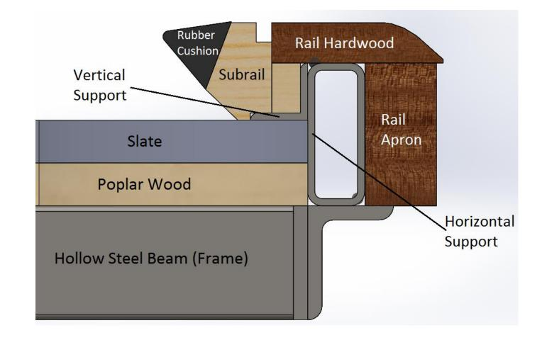
Our frame will be constructed out of steel tubing. The frame supports and secures the slate in both the playing and stowed positions.
