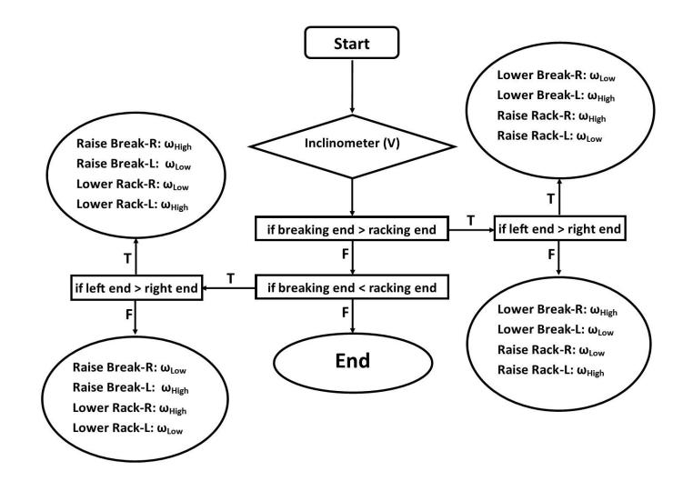
Program logic for the leveling function after the user sets the desired height
