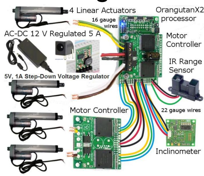
The mechatronic system consists of four 12V linear actuators, a two-axis inclinometer, an infrared range finder, an Orangutan X2 with two Dual motor drivers, an AC to DC converter and a 5V 1A step down voltage regulator.
