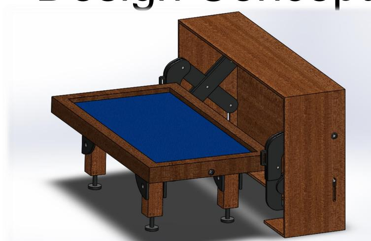
Each leg will be adjustable for the purpose of self-leveling and obtaining the correct height for the stowing process. From there the mechanism rotates the table into its vertical position, which allows it to be pushed into the housing.
