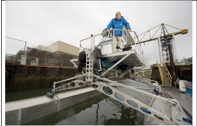
Figure 1. David Hall's self-leveling boat platform iii
