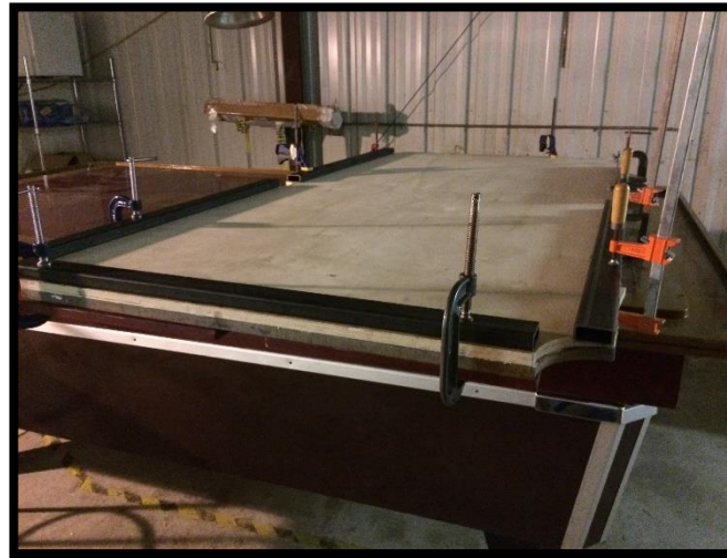
Wood being applied to slate
