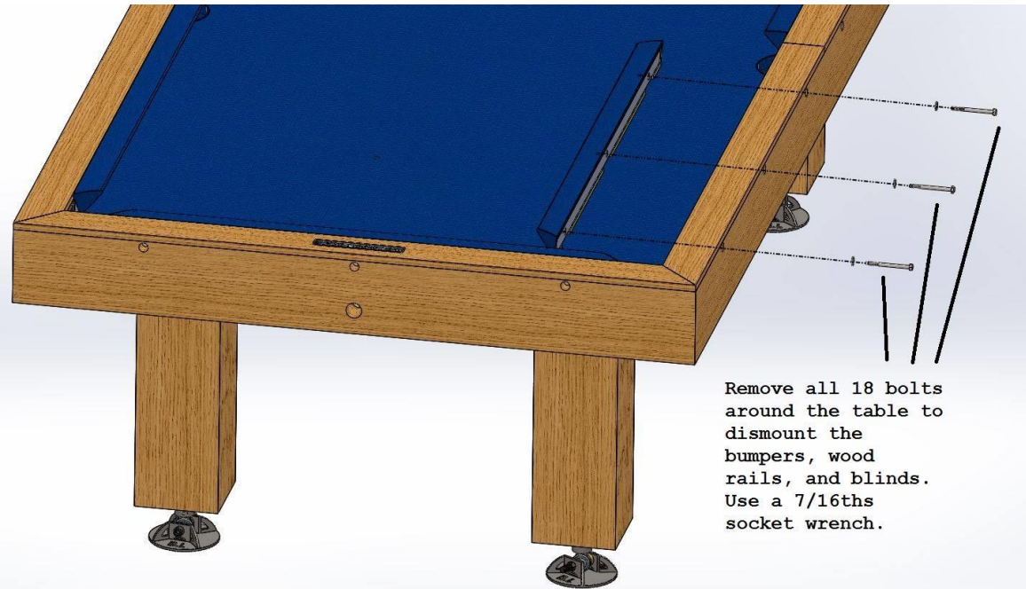
Figure 10. End Bumper Removal (Top) and Side Bumper Removal (Bottom)
