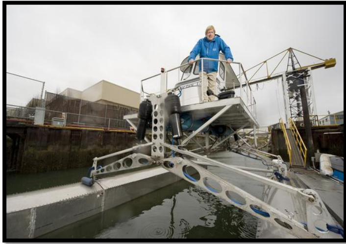
Figure 2. David Hall's self-leveling boat platform
