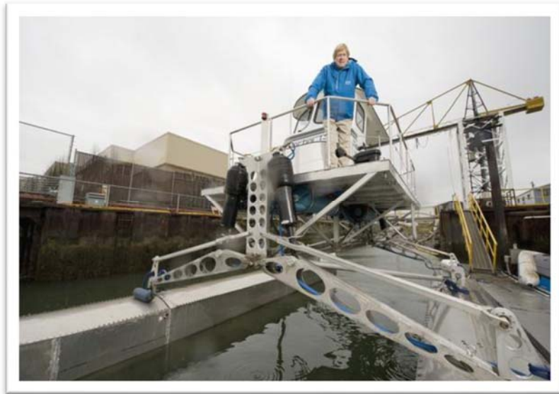
Figure 1. David Hall's self-leveling boat platform [3]
