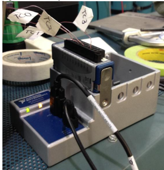
Figure 5. Thermocouple leads inserted into DAQ.
