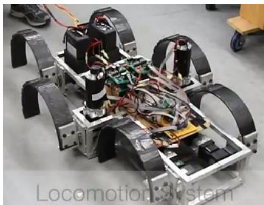
Figure 4 - Synchronized legs following calibration routine.
