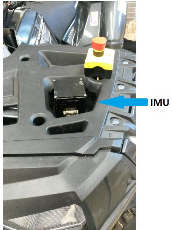
Figure 28. IMU mounting location on the hood of the ATV
