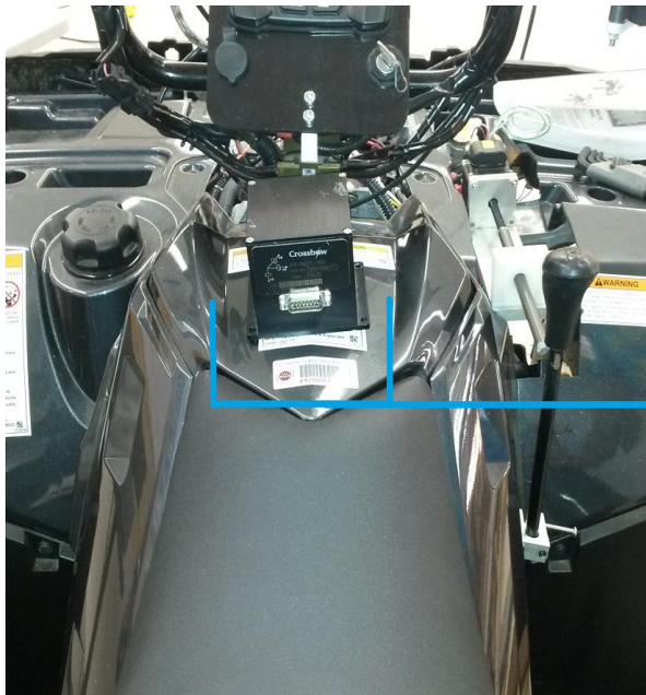
Figure 27. IMU mounting location between handlebars on the ATV's centerline
