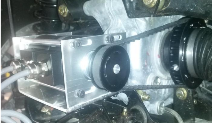
Figure 24: Final mounting for front encoder mounting
