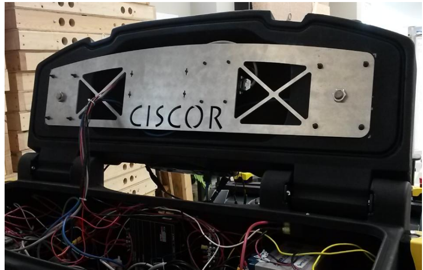
Figure 35: Final mounting of lid plate for GPS, IMU, Router and Antenna
