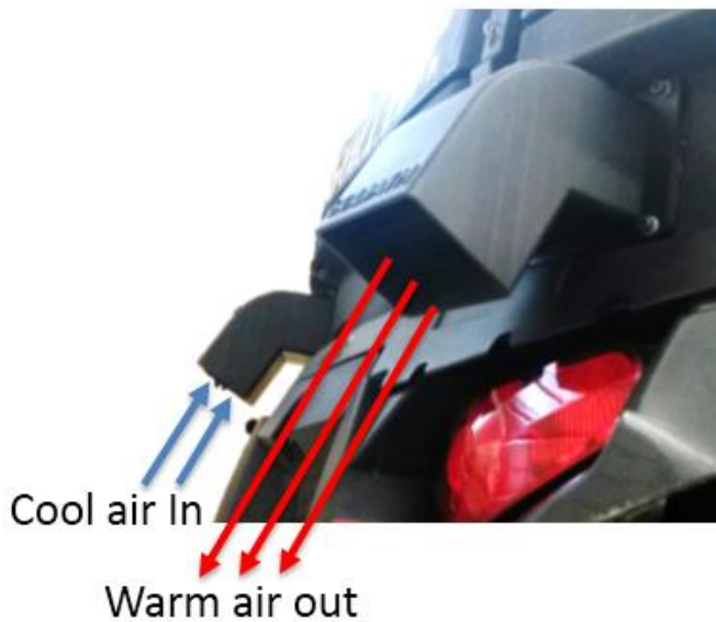
Figure 40: Final snorkel mounting and heat transfer process
