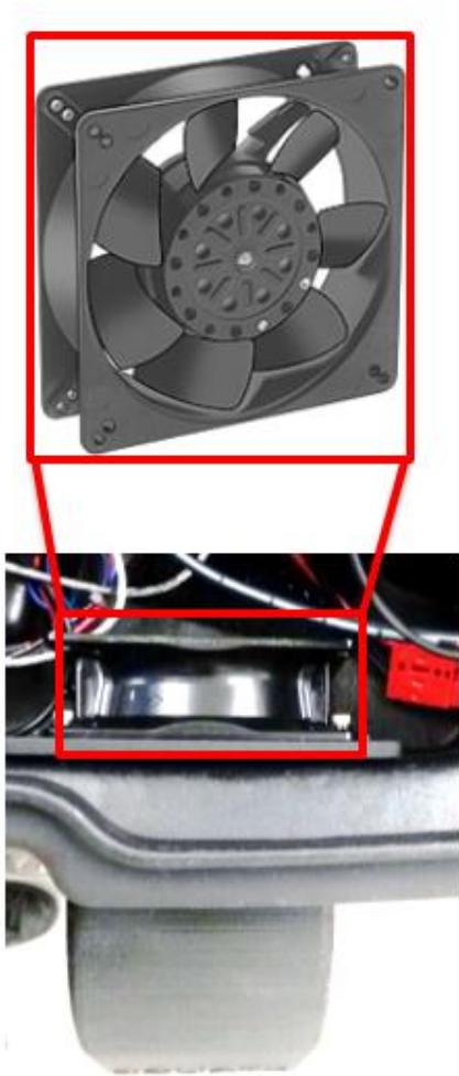
Figure 41: Final snorkel and fan installation
