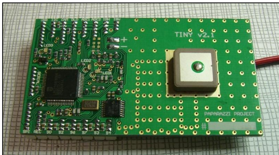
Figure 15- Assembled Paparazzi Tiny (v2.1) autopilot system (26)
