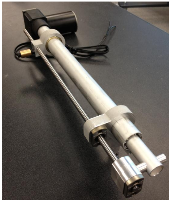
Figure 17 - Z-axis with storage system hardware attached.
