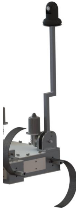
Figure 22 - Camera boom mounted on the rear left corner of the rover.
