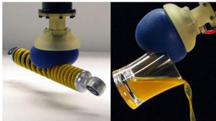
Figure 44: The universal gripper conforms to the shape of any object it is lifting to allow for a delicate yet firm grasp
