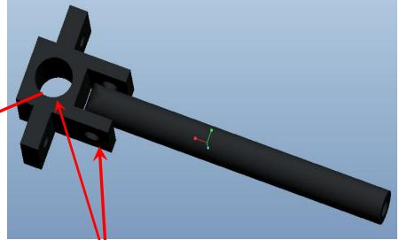
Coupler works as a pin and slider joint to transform an arc into linear motion
