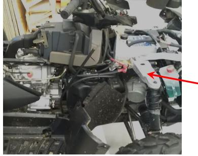
Mount the linear actuator on the body
