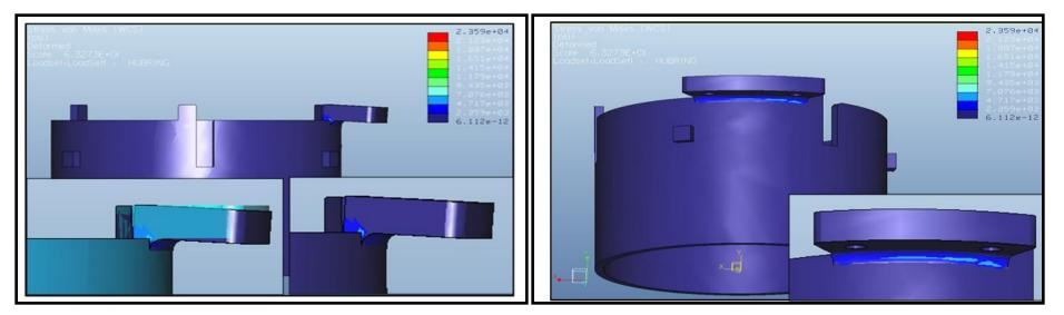
Bottom left most image shows the deformation of the connection tab. Bottom right most image shows the stress concentration point.
