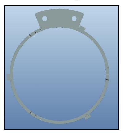
Two threaded holes will be drilled into the tabs in order to secure the panels into place.
