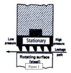
general design of a labyrinth seal is shown in figure 1 [2]. It can be seen that the fluid is prevented from leaking through the seal, by disrupting its flow through the use of turbulent inducing grooves across a very small clearance area. According to Boyce [2], a labyrinth seal has the following advantages: simplicity, reliability, tolerance to dirt, system adaptability, very low shaft power consumptions, material selection flexibility, minimal effect on rotor
